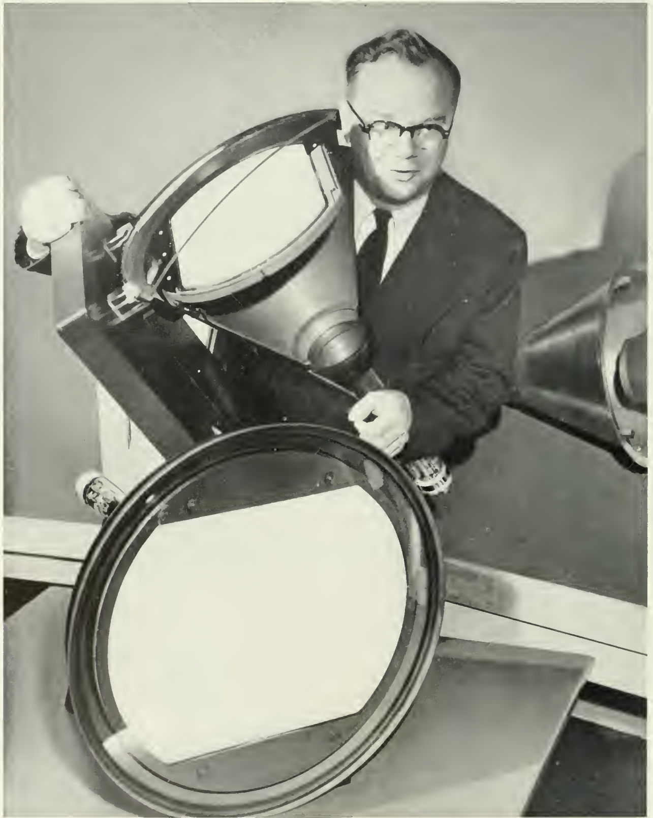
Dr. E. W. Engstrom, Vice President in Charge of Research, RCA Laboratories, holds a model of the 16-inch tri-color picture tube, with RCA's 21-inch tri-color tube in the foreground.
